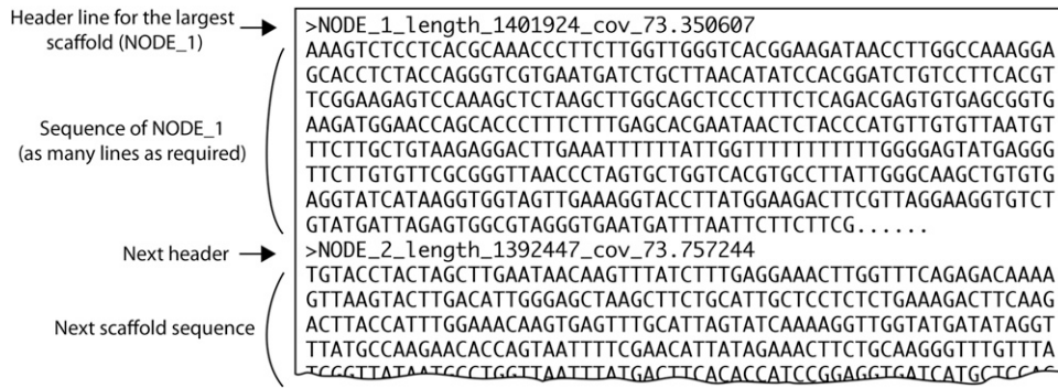
Figure 1 Organization of a scaffolds.fasta file containing a SPAdes genome assembly. The header line for each scaffold begins with a “>” character, which is standard for data in FASTA format. The header for each scaffold shows the scaffold’s node number, its length, and its k -mer coverage. In this example, NODE_1 is 1,401,924 bp long and has 73.35x coverage. The header line is followed by NODE_1’s DNA sequence, and then the header and sequence of the next scaffold (NODE_2). The file can contain thousands of scaffold sequences, one after the other, down to the minimum scaffold size. The scaffolds are always named and sorted in descending order of length.
